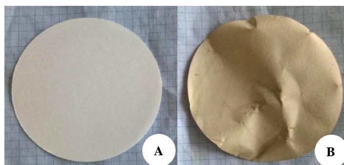
Figure 3. Filter paper: A. No silver nanoparticle coating, B. After silver nanoparticle coating
