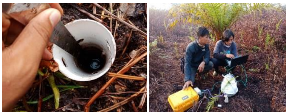
Figure 1. Emission measurement on peatland using the portable Licor-8100
