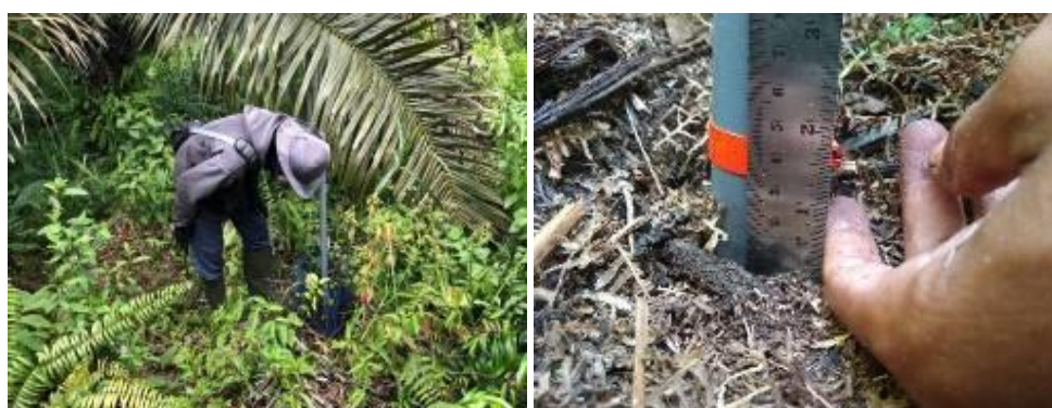
Figure 3. Illustration of measurement of subsidence in small-holder oil palm on peatlands
