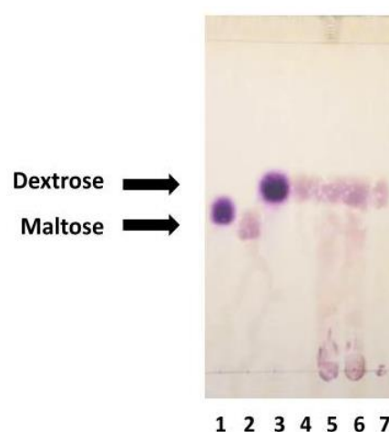
Figure 4. Identification of amylolytic enzyme and its hydrolyzed product using TLC. 1: 1% sucrose, 2: 1% maltose, 3: 1% fructose, 4: 1% dextrose, 5: Hydrolysis of 2% starch by partially-purified enzyme of Aspergillus sp. TM3 PP, 6: Hydrolysis of 2% starch by crude extract of Aspergillus sp. TM3 PP, 7: Hydrolysis of 2% starch by commercial glucoamylase. Starch hydrolysis was done in 60 minutes
