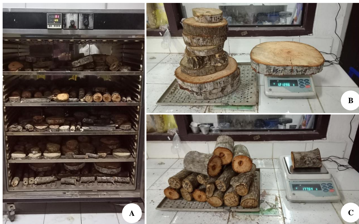
Figure 3. A. The disc and branch samples were dried in an oven, B. The weighing of disk samples of the trunk fraction, C. The weighing of tree branch samples in the laboratory
