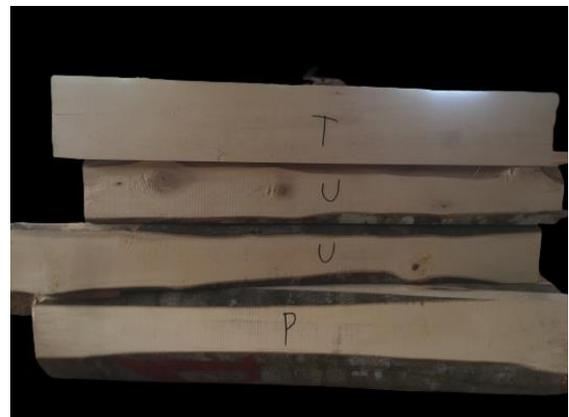
**Figure 1.** Simalambuo wooden beams from the bottom (P), middle (T) and Tip (U)
