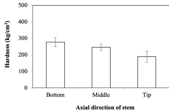
**Figure 8.** The hardness of Simalambuo wood
