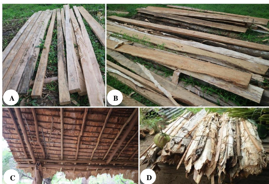
Figure 4. Paperbark trees ( Melaleuca leucadendron ) are processed into various materials. A. Wooden plank blocks 5 x 10 cm, B. Wooden board measuring 2 x 20 cm, C. Wood logs with a small diameter for roof frames, D. Bark for roofing
