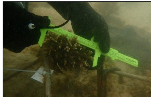
Figure 3. Measurement of coral growth using a caliper
