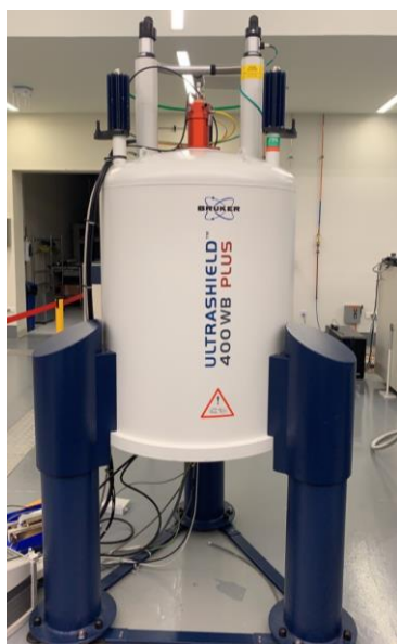
Figure 2. Nuclear Magnetic Resonance (NMR) Bruker Avance III 400 MHz spectrometer
