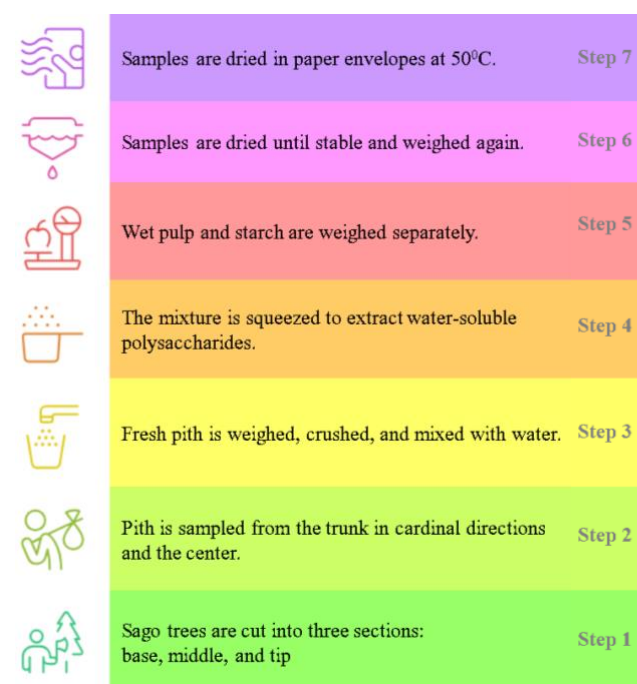
Figure 2. Illustration of preparing sago stem plates as samples
