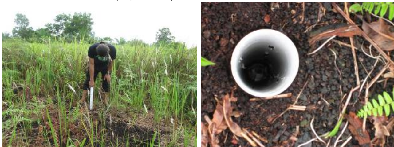
Figure 3. Piezometer measurement and set up in a peatland site impacted by an overflow dam
