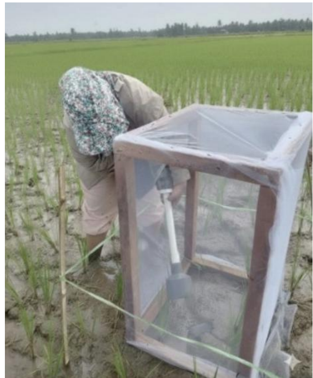
Figure 1. Arthropod sampling using a Farmcop suction sampler in rice fields. The image illustrates the sampling configuration in which rice hills are enclosed in a mesh cage to prevent arthropods from escaping during suction, ensuring standardized, consistent collection from defined sampling units
