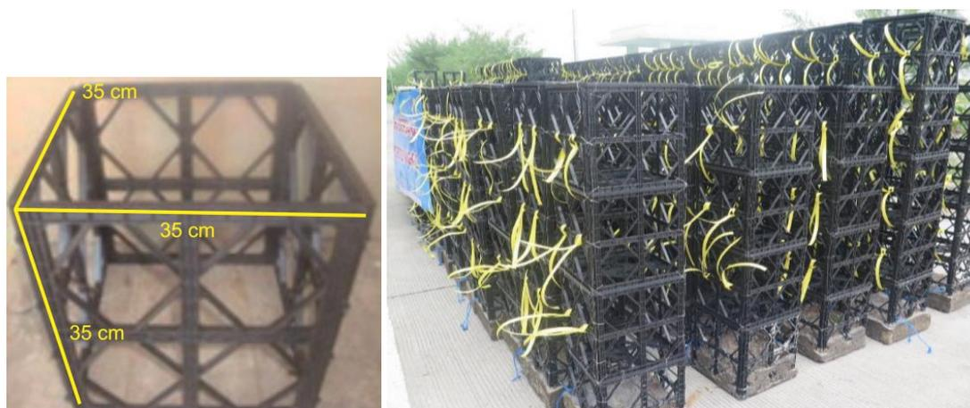
**Figure 2.** Fish apartment partition (*left*), fish apartment design (*right*)
