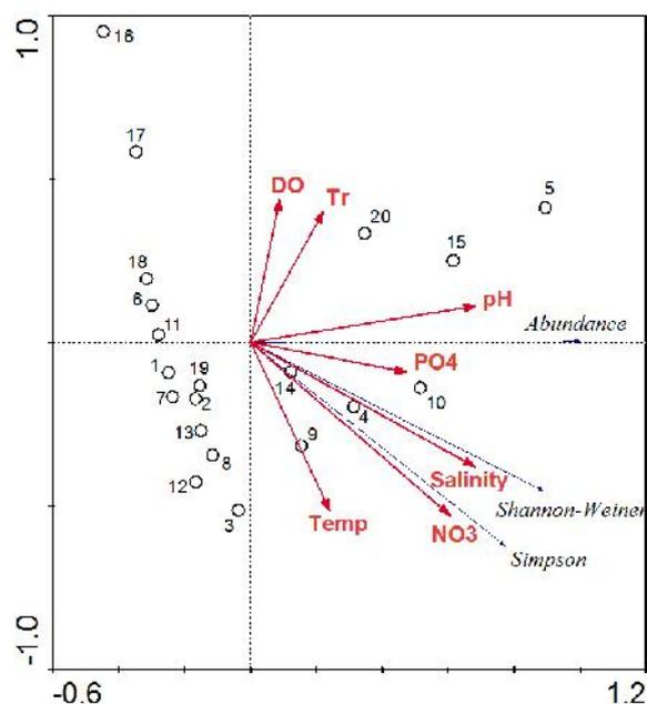
**Figure 5.** Stations-parameters biplot diagram of PCA analysis summarizing the contribution of dominant factors during the study period at different stations. DO (Dissolved oxygen), (pH), Tr (Transparency), Temp (Temperature), (1-5) spring stations, (6-10) summer stations, (11-15) autumn stations, (16-20) winter stations
