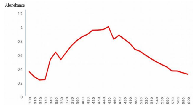
Figure 2. Characteristic peak of silver nanoparticles absorption
