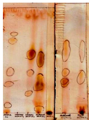
Figure 4.A. TLC card II, C. arietinum leaf fractionation utilizing a fractionating funnel
