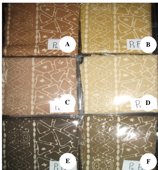
Figure 2. Batik cloth resulted from fixation. Note: A. P 1 F 1 : field location, alum fixator B. P 1 F 2 : field location, calcium oxide fixator, C. P 1 F 3 : field location, ferrous sulfate fixator D. P 2 F 1 : rice field location, alum fixator, E. P 2 F 2 : rice field location, calcium oxide fixator, F. P 2 F 3 : rice field location, ferrous sulfate fixator.
